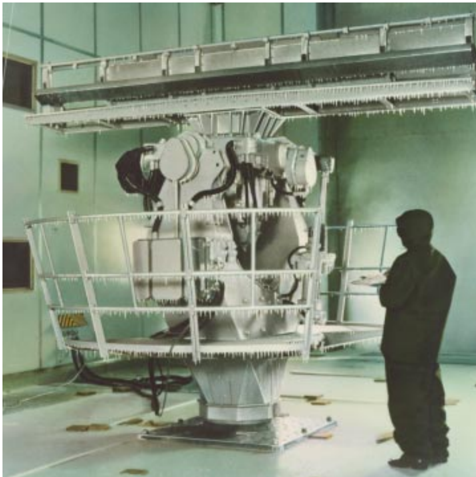
22 Arctic testing of a GWS25 surveillance mount in the Marconi Radar environmental test chamber at Writtle Road
