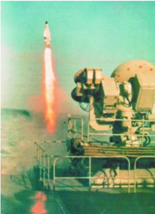
7 SEAWOLF missile tracking radar
